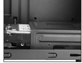
3- Fix the drive to the case body with screws as shown in the picture above
