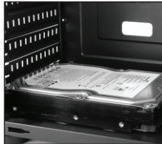
2- Insert the 3.5 inch drive as shown in the picture above
