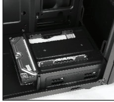
2- Put the desired drive in the bay 3.5 inches
